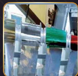
Utilize multiple foil rolls simultaneously, with a maximum of 4 rolls each with a width of 4 inches.
