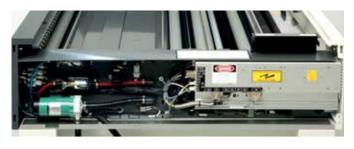
All electronics and mechanical components are located on the sides of the processor, for easy and convenient access during maintenance.
