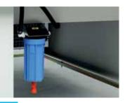
The filter house is conveniently mounted under the frame, allowing access to the cooling unit and extra storage space.
