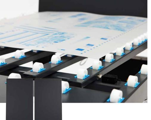
The trolley separates from the PRO Stacker, enabling the stack of plates to be conveniently moved to the press or to storage. The PRO Stacker's conventional stacker design features a belt driven conveyer to transport the plate from the processor to the trolley.
