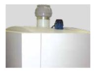
Post-bake oven with extraction heat fan that removes fumes and excessive heat for optimal environmental working conditions.
