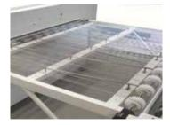
Gentle cooling of plates: Hinged 500 or 1000 mm driven mesh delivery conveyor (optional).
