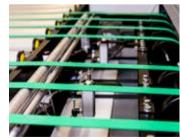
PlateLink 46-XR has a simple belt drive configuration for easy and secure plate transportation.
