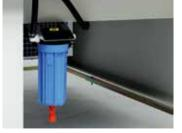
The filter house is conveniently mounted under the frame, allowing access to the cooling unit and extra storage space.
