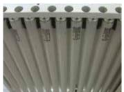
Exposure lamps feature automatic detection of defective lamps, temperature regulation, working hours counter and easy access for replacement.
