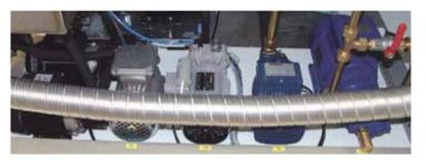
Separate pumps, pneumatic valves and solid content measurement device with dosing pump allows the user to benefit from better solvent condition during use.
