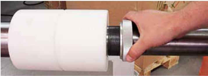
Easily change the adaptor by loosening the ring to remove and replace the adaptor. Please note, that adapters are not included in the standard model, but must be ordered separately.
