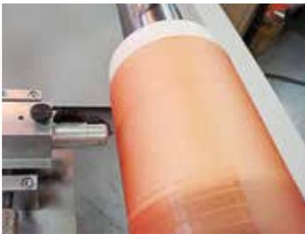
▲ The sleeve is quickly mounted by using compressed air.
